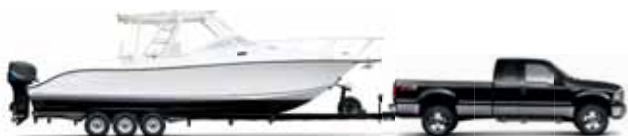
SUPERCAB: MAX. CONVENTIONAL/ MAX. 5TH-WHEEL TOWING F-250/F-350 SRW — Up to 12,500/16,500 lbs. F-350 DRW — Up to 15,000/18,800 lbs.
