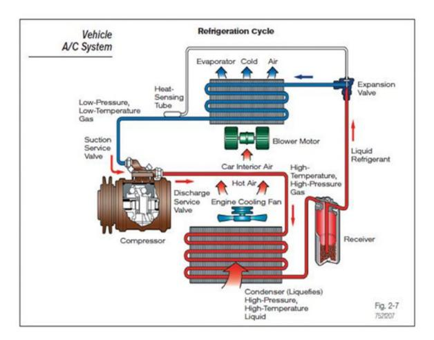
59. As shown below, the Defective HVAC System in the Class Vehicles includes a component called the evaporator, which resides inside the HVAC system module. The system has a high-pressure and a low-pressure side, which includes the expansion valve and the
